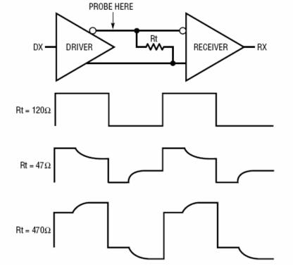
Correct termination resistor that matches the characteristic impedance of the cable is very important in RS485. Otherwise, reflected waves will
