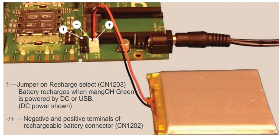
Figure 3-10: mangOH Green With Rechargeable Battery Connected
