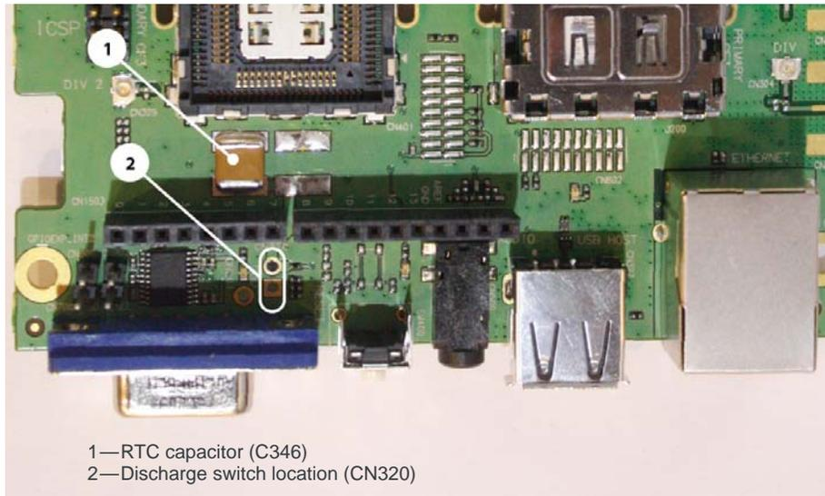
Figure 3-11: RTC Capacitor
