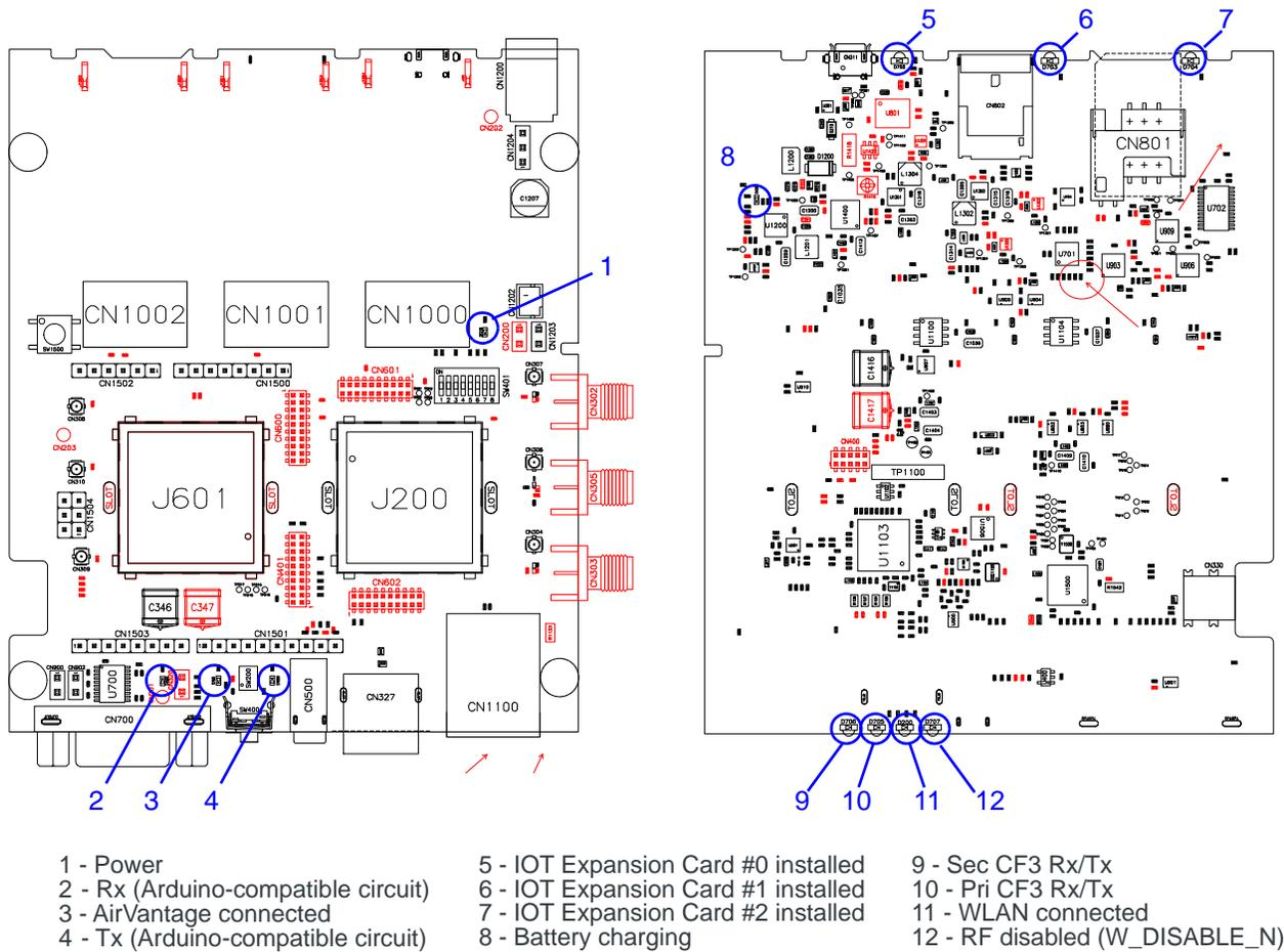
Figure 3-32: LED Indicators (mangOH Green DV4 Configuration)
