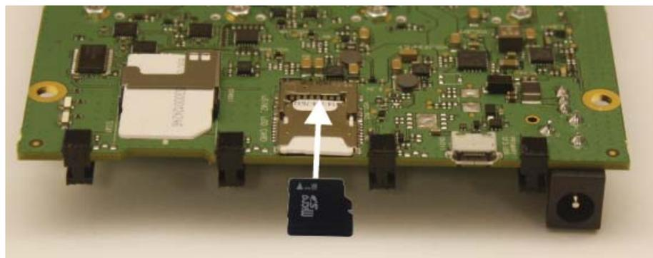
Figure 3-16: microSD—Inserting
