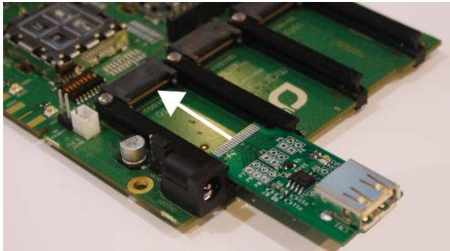
Figure 3-20: IoT Expansion Card Insertion
