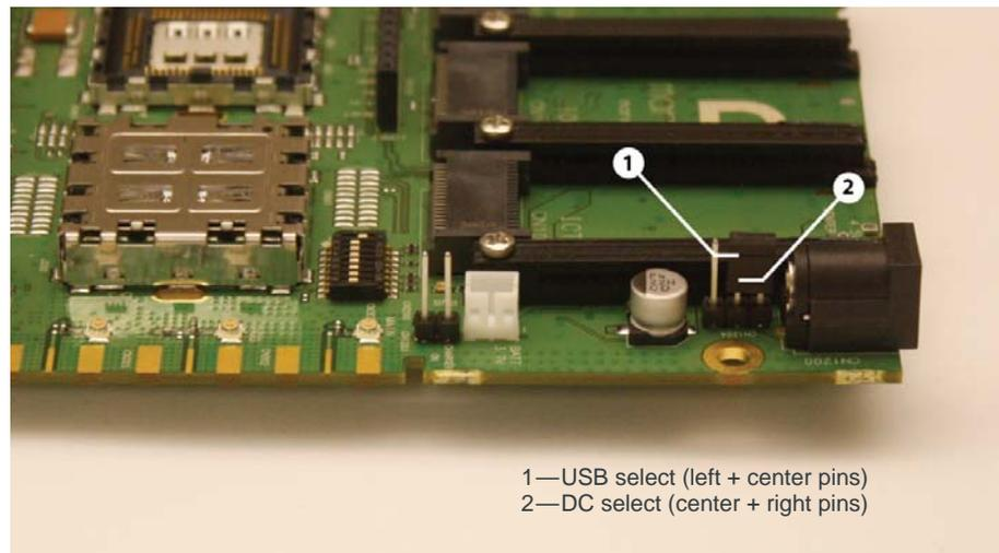
Figure 3-8: Power Source Select (DC power shown)
