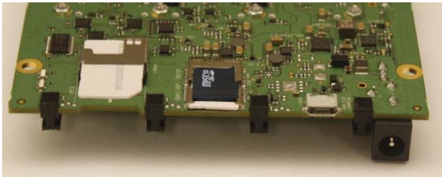
Figure 3-17: microSD—Inserted
