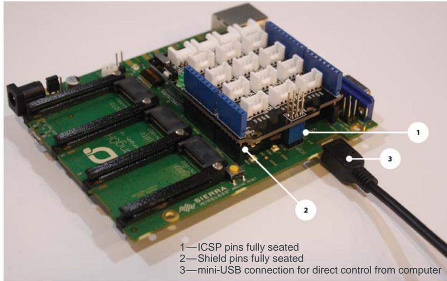
Figure 3-26: Arduino-compatible Shield Installed on mangOH Green
