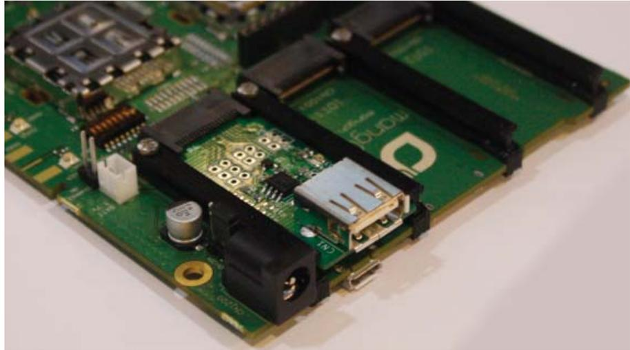
Figure 3-21: IoT Expansion Card Inserted
