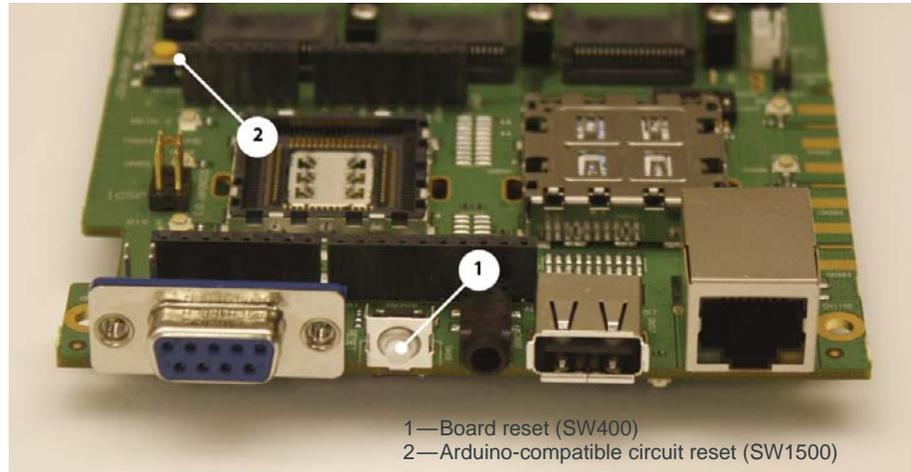
Figure 3-33: Reset Switches
