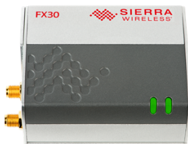
FX30_1104086 Cat M1/NB-IOT Global 75 x 60 x 32 mm
