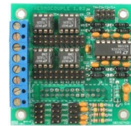
4-channel Thermocouple Board (E,J,K,R,S,T)
