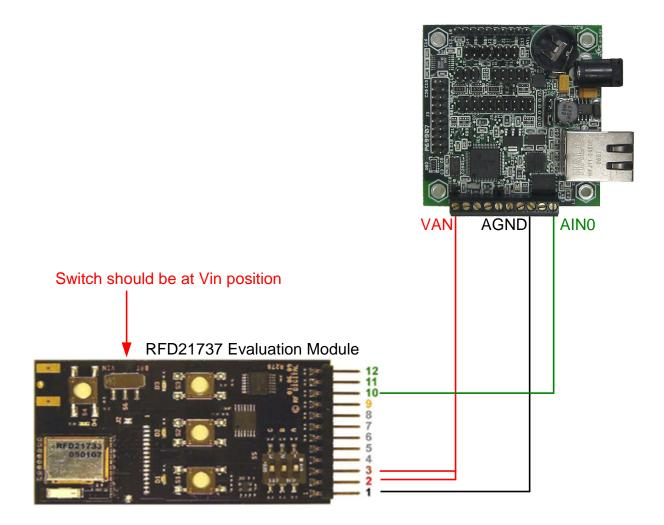
Note: When powering the board from MINI-MAX, the power switch on the board should be on VIN position (NOT on BAT position).
