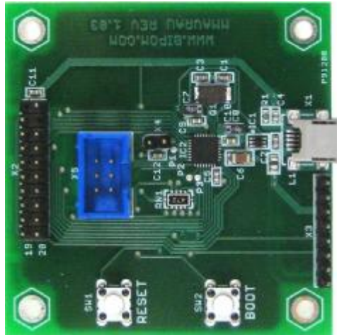
MINI-MAX/AVR-AU General Purpose plus USB support based on AT90USB162-16MU
