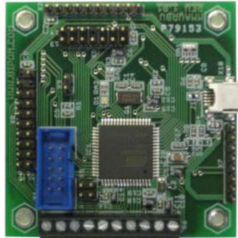
MINI-MAX/AVR-BU General Purpose, USB support, Analog inputs based on AT90USB647
