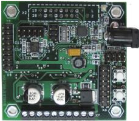
MOTOR-2 Motor Controller based on ATMEGA168V-10
