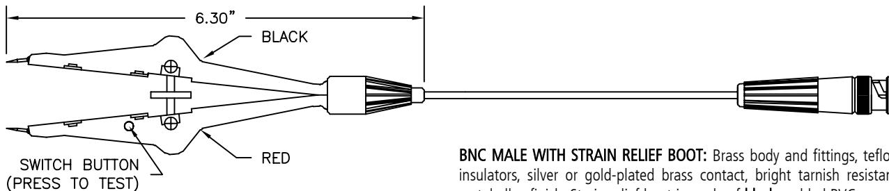
**BNC MALE WITH STRAIN RELIEF BOOT:** Brass body and fittings, teflon insulators, silver or gold-plated brass contact, bright tarnish resistant metal alloy finish. Strain relief boot is made of **black** molded PVC.
