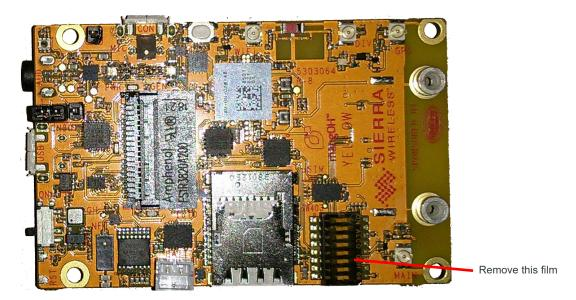
**b.** Make sure all the dip switches are OFF (factory default mode).
