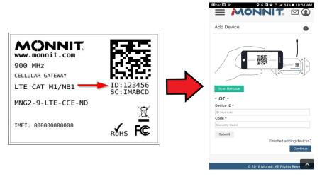
**IMPORTANT:** Add the gateway and all sensors to the iMonnit portal so that on boot, the gateway can download and whitelist the sensors from the account.
