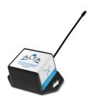
Install a coin cell battery by first taking the sensor and pinching the sides of the enclosure. Gently pull up the enclosure, separating the sensor from its base. Then slide a new CR2032 coin cell battery with the positive side facing toward the base. Press the enclosure back to together; you'll hear a small click.
