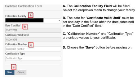
When the new certificate is accepted, the Calibration tab will change to a Certificate tab.
