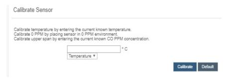
Here you can calibrate the Temperature, 0 PPM, and Upper Span. You can select each of these from the dropdown menu under the text box.
