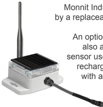
Monnit Industrial Sensors are powered by a replaceable 3.6 V battery (included).
