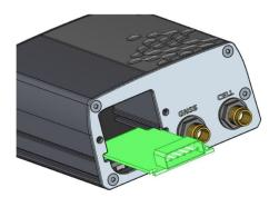
Carefully line up the IoT card with the slots in the aluminium extrusion.
