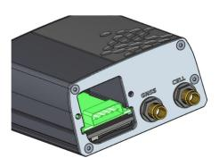
Gently push the IoT card into the slot. There should be almost no force required at this point.
