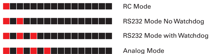
FIGURE 46. Status LED Flashing pattern during normal operation
