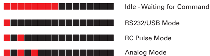
FIGURE 8. Normal Operation Flashing Patterns
