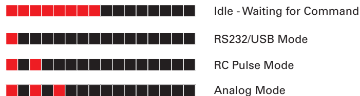
FIGURE 10. Normal Operation Flashing Patterns
