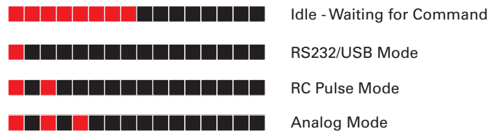
FIGURE 13. Normal Operation Flashing Patterns
