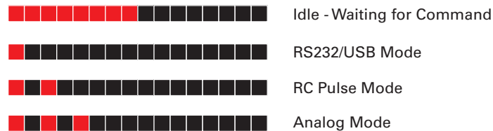
FIGURE 15. Normal Operation Flashing Patterns
