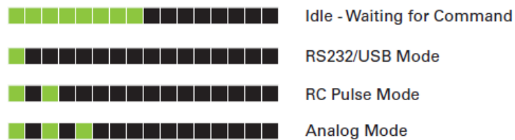
FIGURE 10. Normal Operation Flashing Patterns
