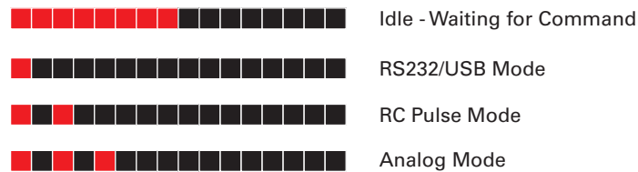
FIGURE 14. Normal Operation Flashing Patterns
