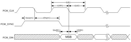
Figure A-2: Timing—PCM Codec to Module
