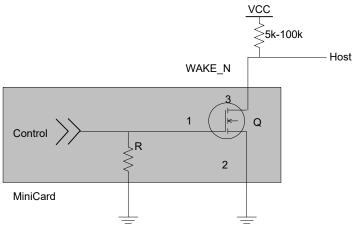
Figure 3-5: Recommended WAKE\_N Connection
