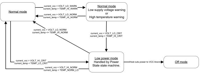
Figure 5-1: Voltage/Temperature Monitoring State Machines
