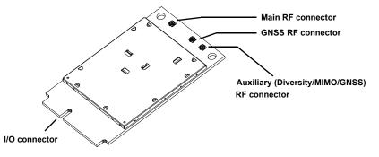
Figure 4-1: Module Connectors
