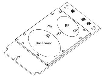
Figure 7-4: Shield locations (Top view)
