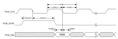
Figure A-3: Timing—Module to PCM Codec
