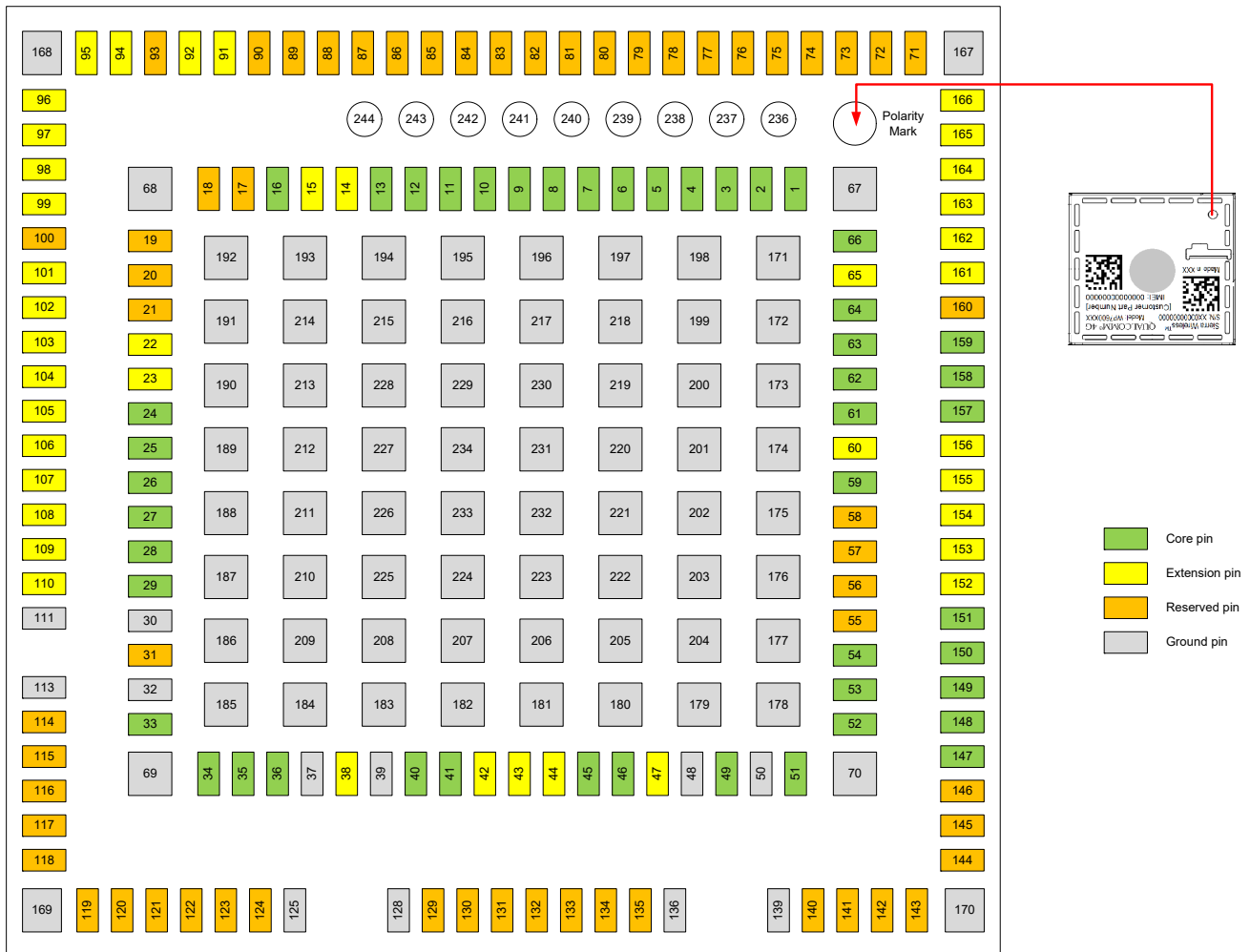
Figure 10-1: Pin Configuration (Top View)
