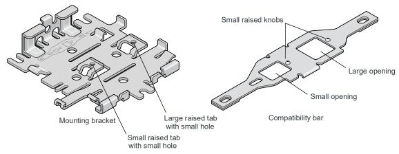
Figure 2-9: Mounting bracket and compatibility bar
