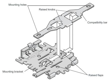
Figure 2-11: Attaching the compatibility bar
