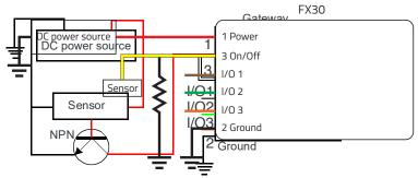
Figure 2-17: On/Off Installation (with sensor)
