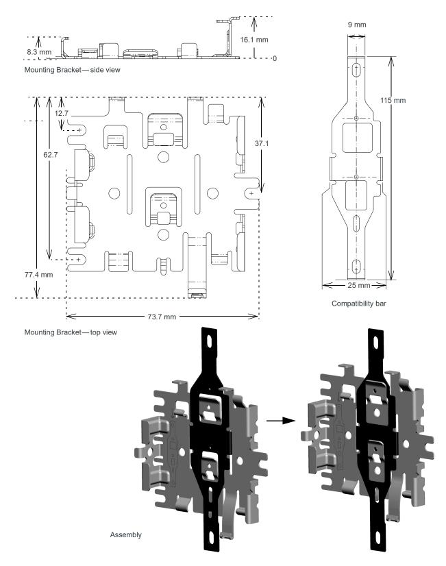
Figure 3-2: Mounting Bracket Mechanical Specifications
