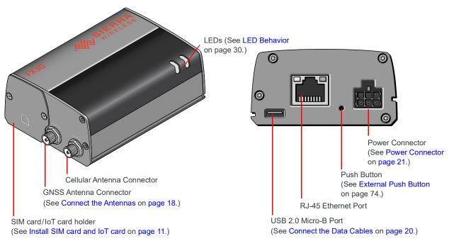
Figure 1-1: FX30 Connectors, LEDs and SIM Card Holder
