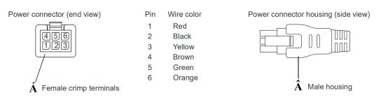
Figure A-1: DC Cable Specifications
