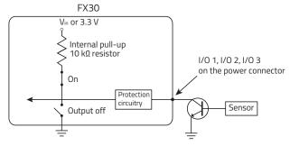
Figure 2-21: High Side Pull-up / Sensor and Transistor Input
