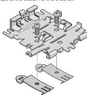
Figure 2-8: Attaching the DIN rail clips
