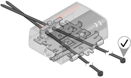
Figure 2-5: Inserting the cable ties
