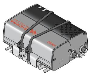
Figure 2-7: Cable ties tightened and trimmed
