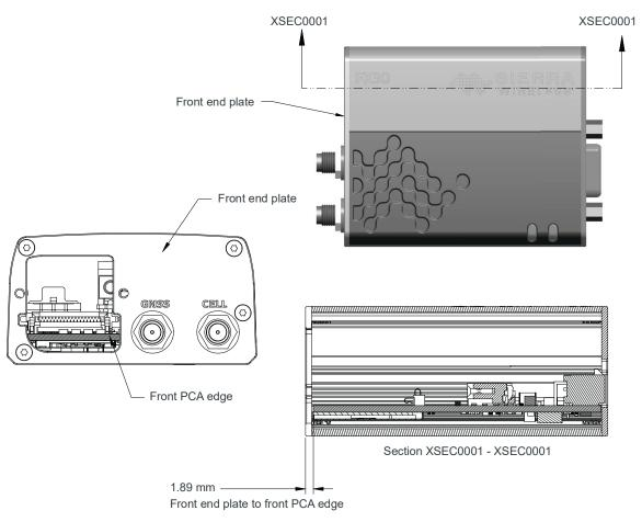
Figure 3-5: IoT Expansion Card Alignment
