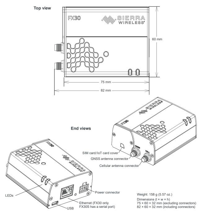
Figure 3-1: FX30 Mechanical Specifications
