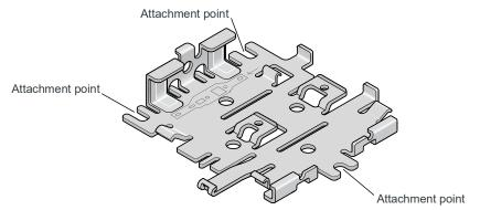
Figure 2-3: Mounting Bracket, showing attachment points
