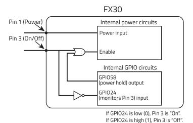
Figure 3-4: FX30 On/Off functionality
