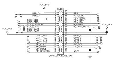
Figure 3-6: IoT Expansion Card Pin Configuration—IoT Expansion Card View
