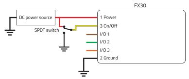
Figure 2-16: On/Off Installation with switch
