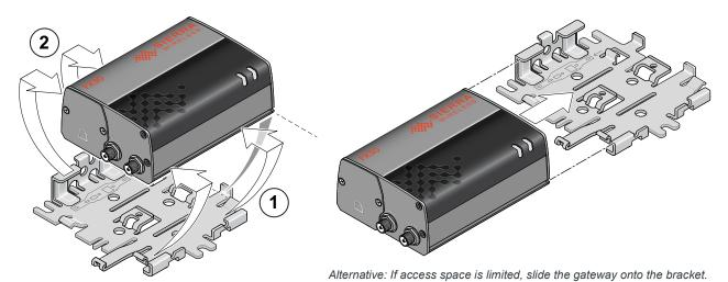
Recommended: Snap the gateway onto the bracket.
