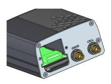
Gently push the IoT card into the slot. There should be almost no force required at this point.
