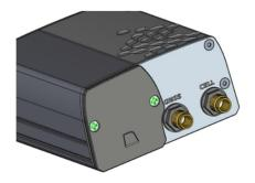
Undo the two countersunk M2 Phillips Head screws and set them aside
