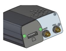
Use the two Pan-Head screws supplied with the IoT card to screw the end-plate into place.
