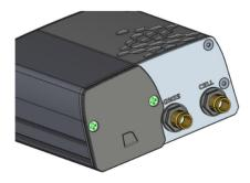
Undo the two countersunk M2 Phillips Head screws and set them aside
