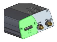
Place the replacement end-plate (supplied with the IoT card) over the end of the connector on the IoT card and line up the two screw holes.
