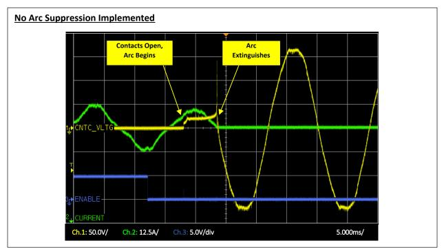
Note that during the 4ms of arcing, the voltage across the contacts is only about 25 to 30V, so a clamping device (e.g., MOV, TVS) would not even be activated during that time.
