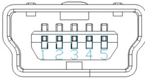
Figure 11: Mini USB Connector
