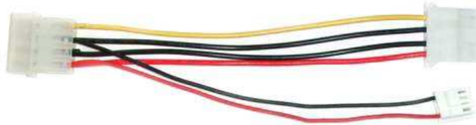
Figure 6: 5V Power Cable
