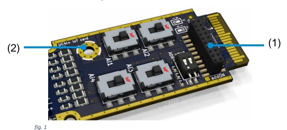
First place the addON card into the slot on the top of the IoT card (1). Then use the polyamide screw (supplied with the addON) to screw the expansion card to the IoT board (2).
