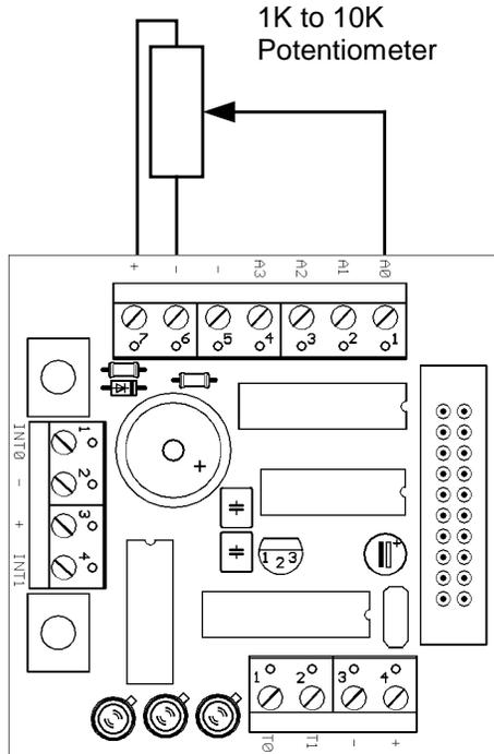
One side of the potentiometer is connected to +5 Volts. The other side of the potentiometer is connected to – ( Ground ). The middle position ( wiper ) of the potentiometer is connected to A0 ( short for Analog 0 ) input of TB-1 board. By rotating the potentiometer wiper, voltages from 0 to 5 Volts can be applied to A0 input.
