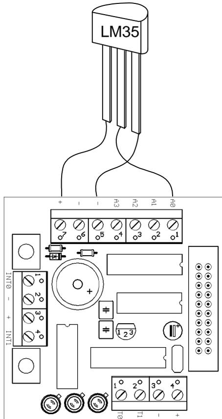
Apply power to MINI-MAX/51-C by plugging the power jack. The program **tb1.hex** should start running and display the voltage values on the terminal window in Micro-IDE. Watch Ch0: ( Channel 0 ). This should show the temperature readings.
