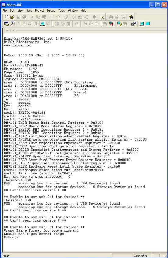
**6.8.** Assign the given MAC address typing the following command on Micro-IDE terminal setenv ethaddr 00:50:C2:46:9x:xx; saveenv
