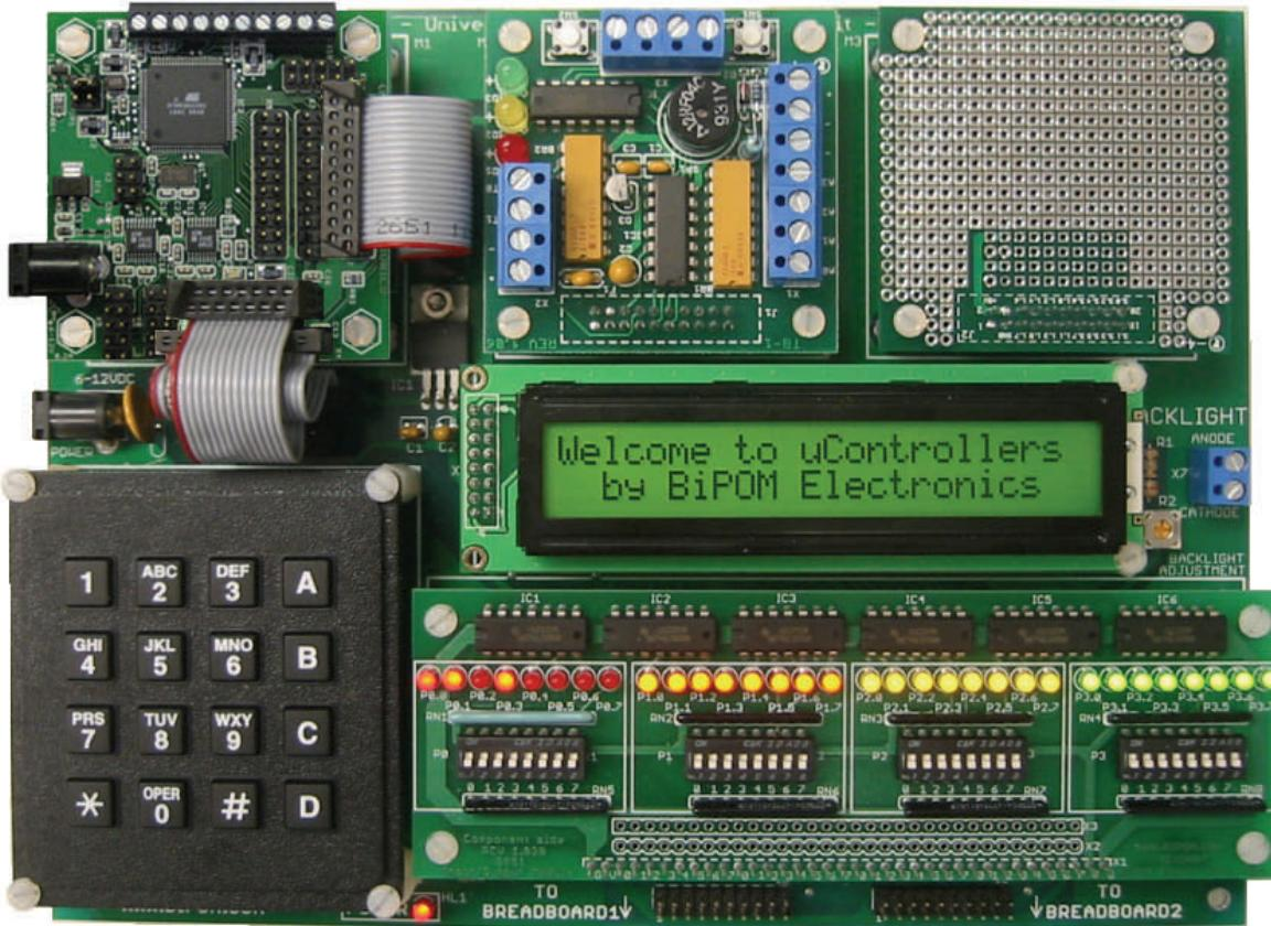
MicroTRAK Supports all BiPOM Electronics **peripheral boards** and includes practical examples for C, BASIC and Assembly Language Programming, Keypad and LCD interfacing, I2C bus, Serial port programming, Motor control, Analog to Digital Conversion and many other fun and instructive projects.
