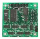
RAM-1: The peripheral memory board for the MINI-MAX and PRO-MAX series of micro-controller systems. RAM-1 has 512Kbyte static RAM and 512Kbyte flash memory with an access via 8-bit address/data multiplexed bus.
