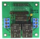
**RELAY-2:** Relay peripheral board with 2 power relays. Normally Open and Normally Closed Contacts.
