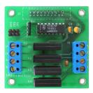
**RELAY-4REED:** Relay peripheral board with 4 reed relays. Normally Open Contacts.
