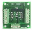
**DAC-1** and **DAC-2** are 8-bit Digital to Analog Converter (DAC) boards with I2C 2-wire interface. DAC-1 has 4 analog output channels. DAC-2 has 8 analog output channels. All outputs and their corresponding ground returns connect to screw type terminal blocks.
