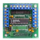
**DAQ-127** and **DAQ-128** are 8-channel, 12-bit, Analog Input and 1 channel, 10-bit Analog Output peripheral board. DAQ-127 has +/- 10 Volt input range. DAQ-128 has +/- 4 Volt input range.
