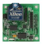
**CB-1** is a wireless communications peripheral board for the MINI-MAX series of microcontroller systems. CB-1 provides Infrared, Zigbee, Bluetooth communications for a host microcontroller.
