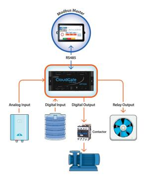
In this mode, CloudGate IO Box will act as a Modbus RTU slave based on the RS485 interface connected. Various devices can be connected over the Analog and Digital I/O of the CloudGate IO Box.
