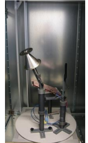
Bluetest Reverberation chamber (antenna efficiency, diversity gain, TIS, TRP)
