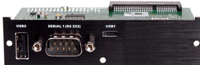
Figure 1: Telematics base board.
