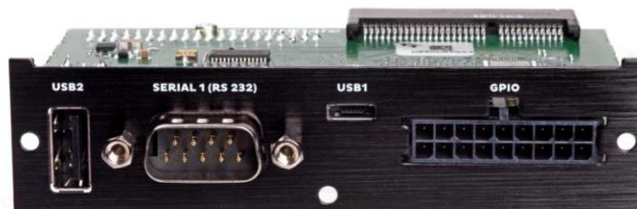
Figure 3: Telematics card with CAN I/O expander.
