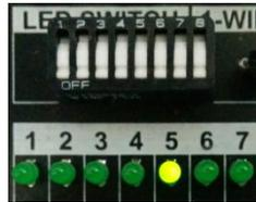
Figure 30: Switch on "ON" position and LED number 5 ON.
