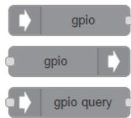
Figure 28: GPIO nodes.
