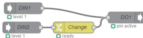
Figure 47: Final configuration using Digital inputs for one output.
