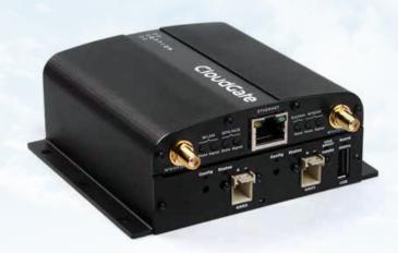
The KNX Card provides the CloudGate with a TP1 interface to a KNX installation. It can also accept a range of Option or third party developed I/O expanders that match the card to specific applications.
