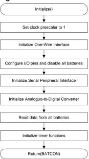
The initialisation function always exits with the same return code, pointing to the state function for battery control.
