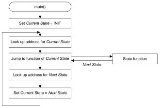
Upon return, the state machine expects the function to indicate the next state as a return argument. The recognised return codes are described in the table below.
