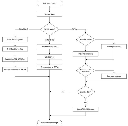
Figure 4-13. Flow chart of USI overflow interrupt service routine.
