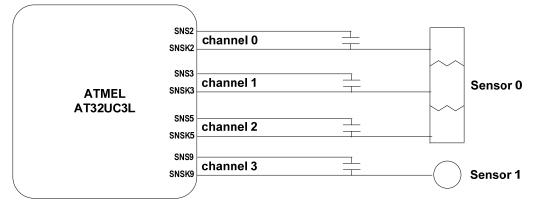
Figure 41 QTouch method Channel/Sensor numbering
