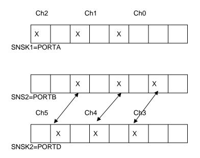
This example is for intraport-interport 12 channel library with two port pair used. Channel0 is A1A3,Channel1 is A4A5 and Channel2 is A6A7 are enabled in the first port pair. Channel3 is B1D2,Channel4 is B3D4 and Channel5 is B5D6 are enabled in the second port pair.
