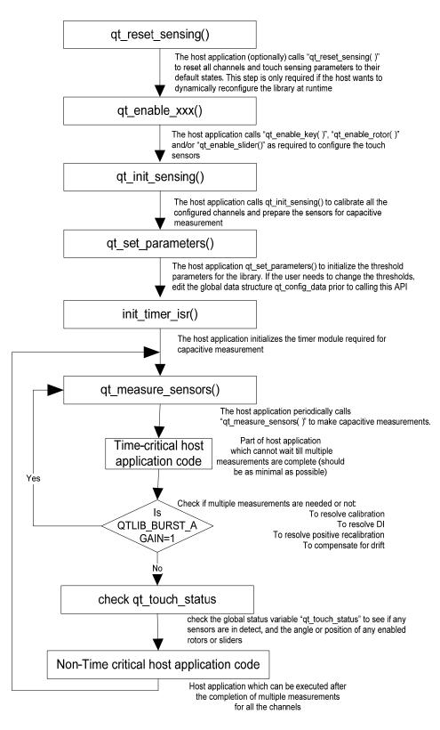
Figure 5-6: Sequence of operations to add Touch capability
