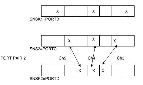
This example is for interport-interport 16 channel library with two port pair used. Channel0 is A2B0,Channel1 is A4B3 and Channel2 is A5B6 are enabled in the first port pair. Channel3 is C1D2,Channel4 is C3D3 and Channel5 is C5D4 are enabled in the second port pair.
