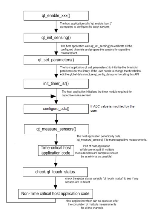
Figure 52 QTouch method for Tiny40 API Flow diagram
