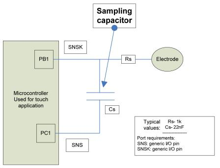
Rs- Series resistor, Cs - Sample capacitor, PB1- PortB bit1, and PC1- PortC bit1
