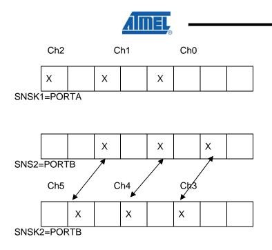
This example is for intraport 8 channel library with two port pair used. Channel0 is A1A3,Channel1 is A4A5 and Channel2 is A6A7 are enabled in the first port pair. Channel3 is B1B2,Channel4 is B3B4 and Channel5 is B5B6 are enabled in the second port pair.
