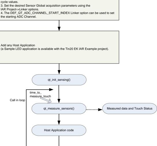
Figure 50 QTouch method for Tiny20 API Flow diagram
