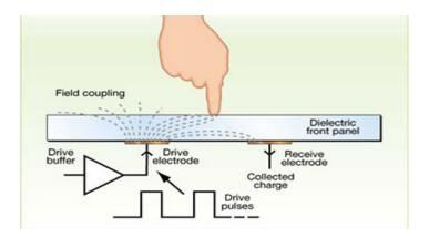
Figure 5-4 : QMatrix Acquisition method
