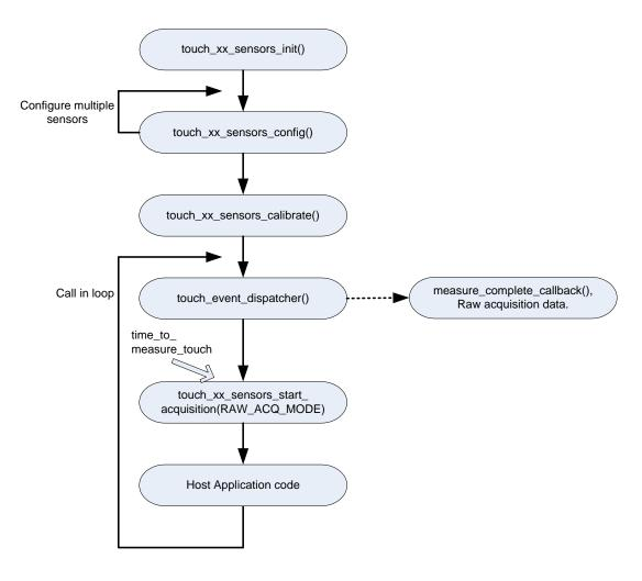
Figure 45 Raw acquisition mode API Flow diagram
