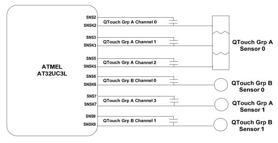
Figure 42 QTouch method Channel/Sensor numbering when Group A and B are used together
