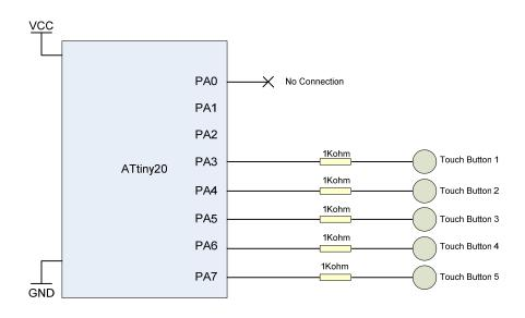
Figure 48 Schematic overview of QTouch on Tiny20
