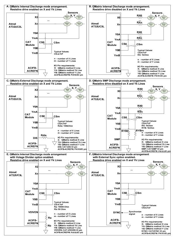
Figure 37 QMatrix method schematic
