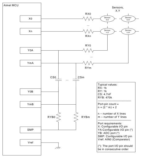
Figure 5-5 : Schematics for a QMatrix acquisition method design
