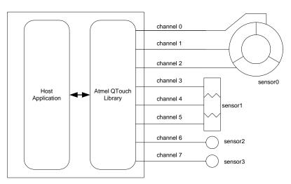
Figure 5-1 : Typical interface of the ATMEL QTouch library with the host application.
