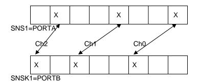
This example is for interport 8 channel library with only one port pair used. Channel0 is A0B2, Channel1 is A3B5 and Channel2 is A7B7 are enabled for the 8 channel library.
