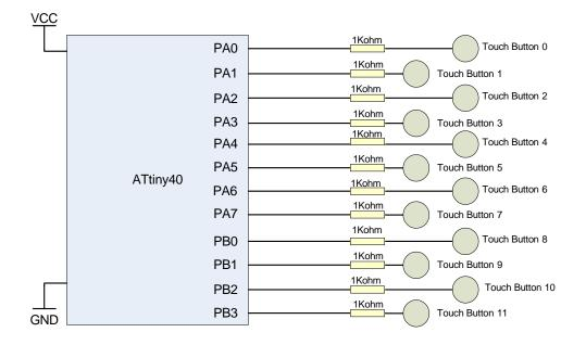
Figure 51 Schematic overview of QTouch on Tiny40
