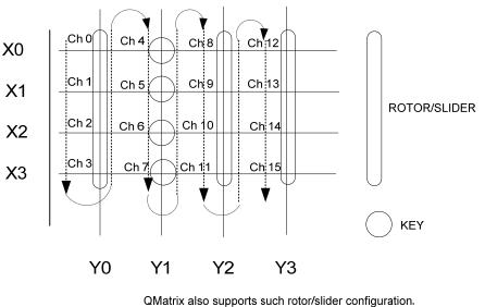
QMatrix Channels The channels selected for a Rotor / Slider MUST be on a single YA/YB line.
