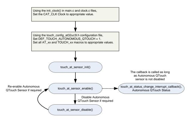
Figure 44 Autonomous QTouch API Flow diagram
