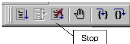
When debugging is stopped, all debugging related windows such as Register window, Memory window and Variable window are automatically closed.
