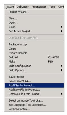
Select test.asm from c:\test to add to the project:
