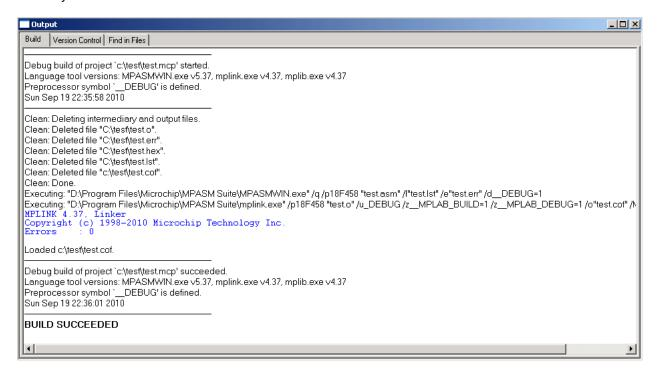
The successful build generates several files, including *test.hex* which is the output file that will be downloaded to the MINI-MAX/P18 board.
