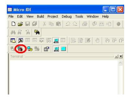
• Press "Program Target Device" to download the code to the target MINI-MAX/P18 board:
