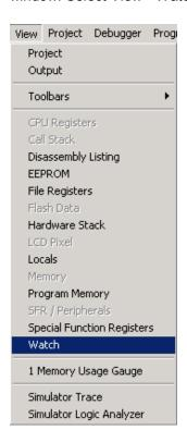
This will open Watch window. Select the Special Function Register to be watched from the left pull down list. In this case, we are using PORTC in our program so we can watch the value of PORTC:
