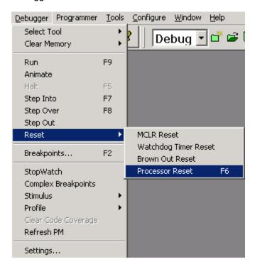
This will reset the simulated microcontroller and place the current program position indicator ( Program Counter ) on the first executable line of code:
