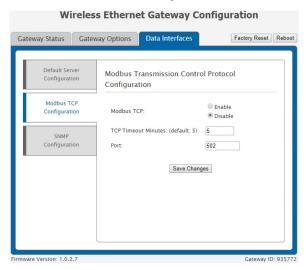
Modbus TCP interface runs on an Ethernet connection. TCP makes sure all data is received. Modbus TCP is a non-streaming data interface standard. This means data must be requested in order for it to be received. The Modbus TCP Interface will store all data values in 16-bit registers. The registers and their associated data fields are mapped below.
