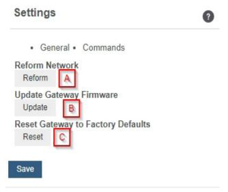
**A.** Selecting the **Reform Network** command will trigger the gateway to remove all sensors from the internal whitelist, and then request a new sensor list from the server. This command will force all sensors to reinitialize their connection with the gateway.
