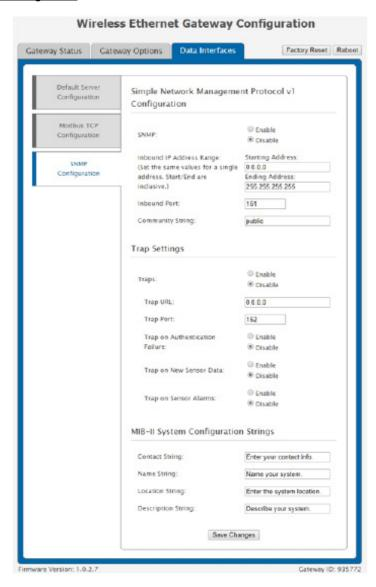
SNMP (Simple Network Management Protocol) settings for a gateway can be adjusted on the offline local interface. You can continue to use SNMP without the server interface active. The data will not be sent to a server, but you can continue to poll for the data as it is received by the gateway.
