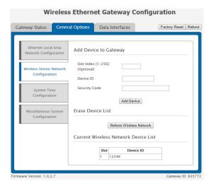
**Slot Index** - The slot index is an optional setting for assigning your gateway. If a Slot ID is entered, the device will be added to the appropriate slot in the Wireless Device List. If a slot ID is not entered, the device will be added to the first available slot.
