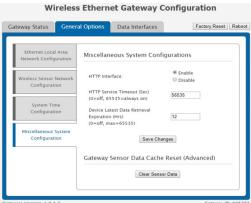
HTTP Service Timeout: This is a security setting for allowing this web interface to be active. The default is 5 minutes. Setting the field to 0 will turn it off
