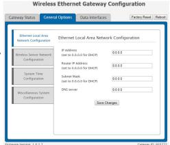
**DNS Server -** DNS Servers take alphanumerical data (like a url address) and return the IP address for the server containing the information you're looking for.
