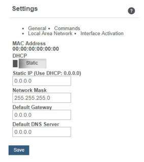
**Static IP** - A static Internet Protocol (IP) address is a numerical sequence assigned to a computer by a Network Administrator. This is different from a Dynamic IP Address in that a Static IP doesn't periodically change and remains constant.
