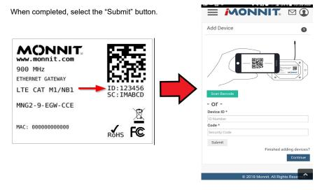
**IMPORTANT:** Add the gateway and all sensors to the iMonnit portal so that on boot, the gateway can download and whitelist the sensors from the configured sensor network.
