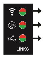
Steady Green: Communication with sensors is normal. Blinking Green: Active communication with sensors. Steady Red: Gateway hardware may be faulty
