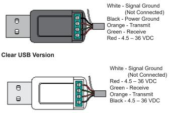
Note: The white wire is not used with the USB programming dongle. The white should be left unconnected but protected to prevent accidental shorting.
