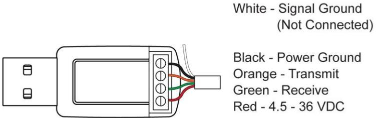
**Note:** The white wire is not used with the USB programming dongle. The white should be left unconnected but protected to prevent accidental shorting.
