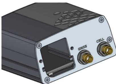
After removing the end-plate, the IoT slot (and SIM slot) can be accessed
