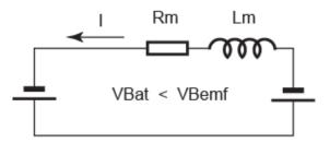
Fig 5: Regenerative braking condition
