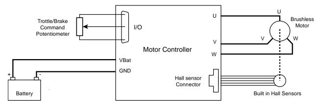
Fig 8: Motor connection of Roboteq motor controller
