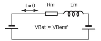
Fig 4: Stable speed without load or friction
