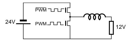
Fig 6: Step down conversion at 50% PWM
