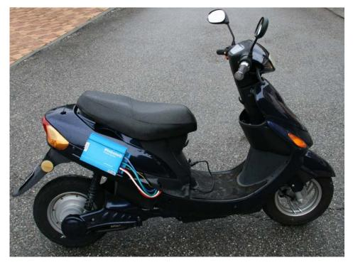
Experimental electric scooter capable of progressive regenerative braking using Roboteq Brushless motor controller
