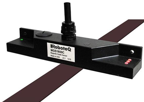
In this application note, the AGV will follow a track made of an adhesive magnetic tape affixed on the floor. The MGS1600C will measure the how far from the center of the tape it is and provide the
