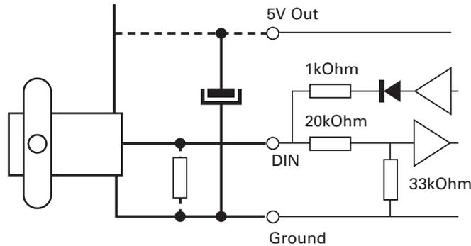
FIGURE 8. RC Servo wiring
