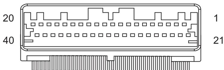
FIGURE 3. MX34 connector pin locations
