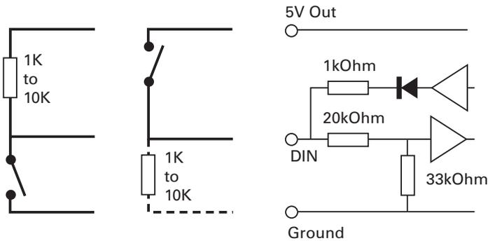
FIGURE 6. Pull down and Pull up switch wiring
