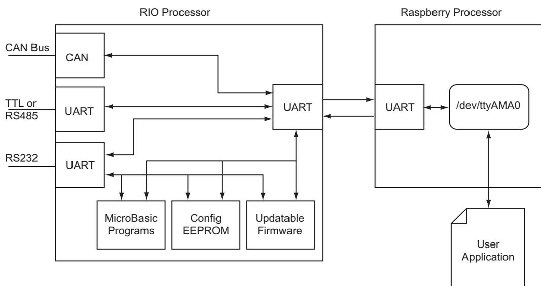
FIGURE 11. Serial Communication between RIO and Raspberry Pi
