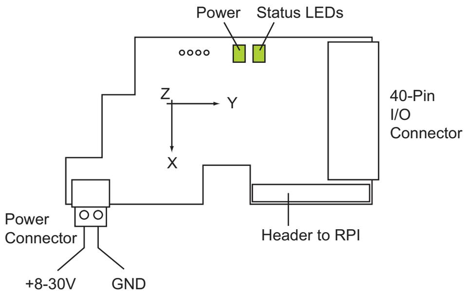
FIGURE 2. RIO board connectors and status LEDs
