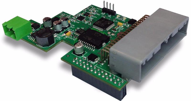
Roboteq's RIO (Raspberry IO) is an intelligent I/O expansion card that is designed to turn Raspberry PI into a powerful and inexpensive embedded computer for robotics navigation, unmanned vehicles, machine control, industrial & home automation and any other applications that need interfacing to the real world.
