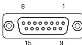
FIGURE 12. Connector pin locations
