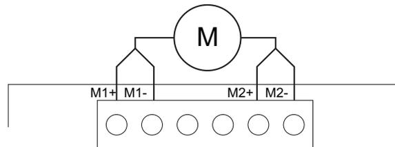
FIGURE 11. SDC2130S and SDC2150S wiring diagram
