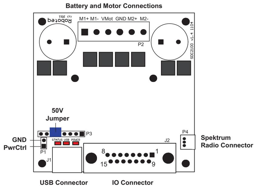
FIGURE 8. Controller layout
