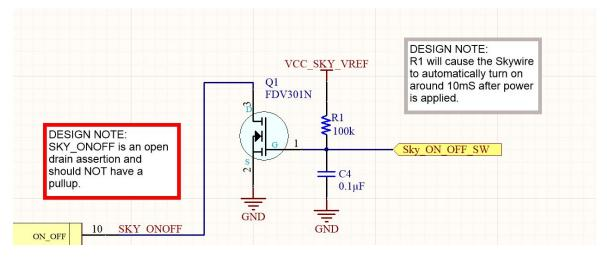
To initiate the startup procedure, tie ON OFF to ground for at least 1 second.
